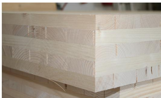
**Figure 1: Cross-laminated wooden panel**
