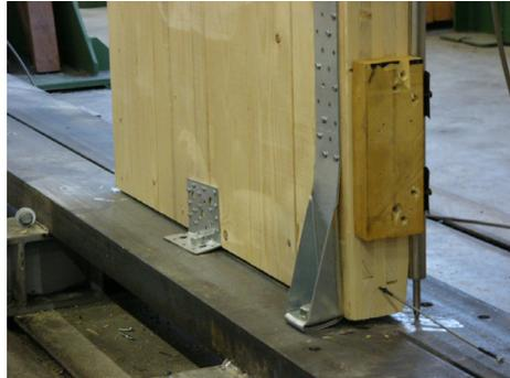
**Figure 12: rigid panel with gap (D/1b)**
